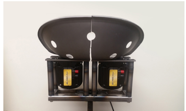
Split seat with dual vibration drives on a chair. Independently-controlled vibration sources are mounted to the underside of the seat.
