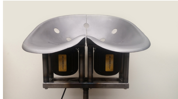
Split seat with dual vibration drives on a chair. Independently-controlled vibration sources are mounted to the underside of the seat.
